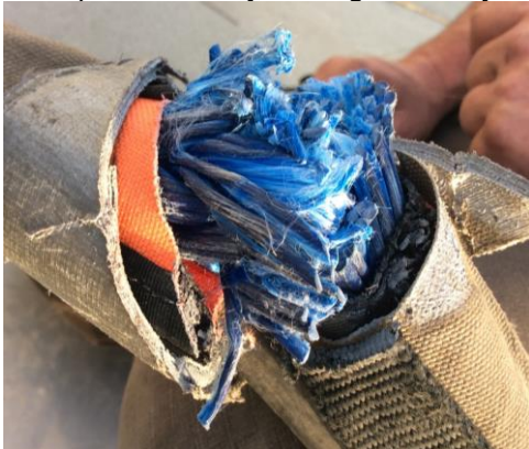
Example of a heavy-lift longline cut by a kite line:
