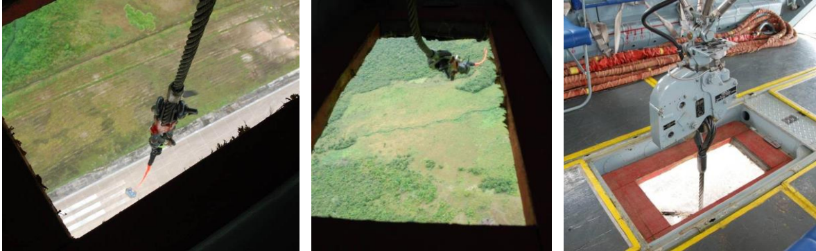
Example of a steel lanyard through a cut-out hole on a Mil Mi-171:
