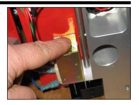
Adjust the position of the control rod so that the locking pin on the open solenoid aligns with the groove in the feed control rod.
