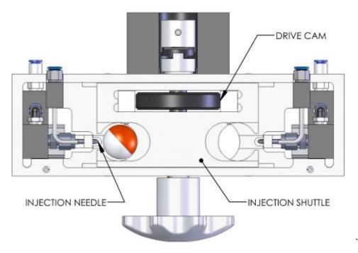
Outward motion of the shuttle causes the sphere to contact the injection needle and be injected with glycol. For details of the injection process, see *Section 3: Glycol System*.
