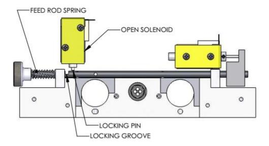
When the close solenoid is energized, it pushes the feed control rod inwards, causing the feed gates to block the flow of spheres through the passages. The spring loaded pin re-enters the groove in the feed control rod and locks the gates closed. In an emergency, the feed gate can be closed and locked by pushing the manual feed gate knob located on the end of the feed control rod.
