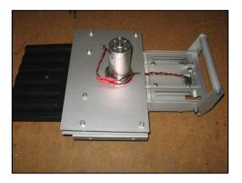
• Loosen the # 8-32 setscrew which secures the agitator cam to the hopper motor shaft.
