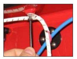
• Remove the three # 10-32 x 3/8 seal screws that secure the level switch into the tank.
