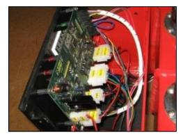
• Remove the nut on the front of the panel which secures the circuit breaker.
