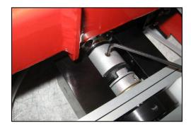
• Remove the two #10-32 x 1-3/4 socket head capscrews which secure the motor mount to the injection head.
