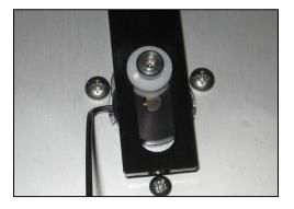
• Replace the agitator mechanism into the hopper body and secure using four # 10-24 x 3/8 button head capscrews.
