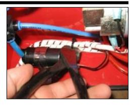
Attach the new pump wiring harness to the pump ensuring that the red lead is attached to the positive terminal
