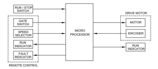
When the "RUN / STOP" switch is in the "STOP" position, the inputs from the remote control are ignored and the drive motor will not run. When the gate switch is pressed to the "OPEN" position, a signal is sent to the gate solenoids to open the feed gates. After a short delay, a signal is then sent to turn on the drive motor.
