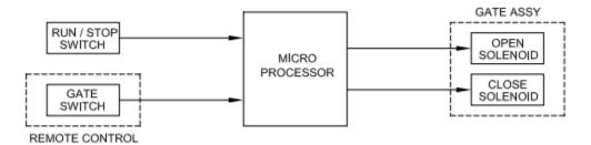
When the "RUN / STOP" switch is in the "STOP" position, the inputs from the remote control are ignored. When it is switched to the "RUN" position, there is also a short delay before the remote control signals are acted upon. This is to ensure that the hopper has time to fill its outlet queues before the gates open.
