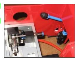
• Replace the check valve ensuring proper orientation.
