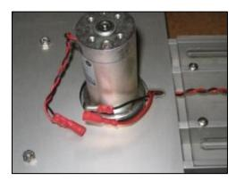
• Align the motor shaft flat with the setscrew in the agitator cam and tighten the setscrew.
