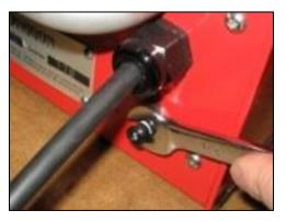
Disconnect the power wiring harness from the main circuit breaker.
