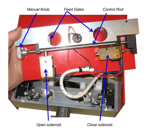
As the spheres exit the hopper, they enter two vertical passages in the feed gate assembly. Each passage has a feed gate attached to a common control rod. Pushing the rod inwards causes the feed gates to block the passages and stop the flow of spheres.
