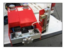
• Unlock the feed gate control rod by lifting up on the open solenoid plunger with a slotted screwdriver. The feed gate control rod should spring open.
