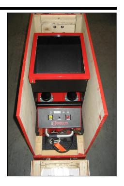
• Place the support base in the crate between the hopper and the open end above the control panel.
