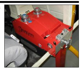
Pass the free end of the strap beneath the belly of the aircraft and in under the opposite door. Check that the strap is not twisted or obstructing any aircraft vents, antennae or release cables. Feed the free end up and over the roller on the quick release fitting attached to the other end of the dispenser. Pull the free end to tighten the strap.
