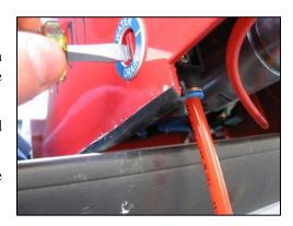
• Remove the feed gate assembly.
