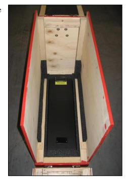
• Place the main body of the dispenser into the crate with the control panel facing the open end of the crate.
