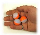
The Red Dragon injects a constant volume of glycol into each Dragon Egg regardless of the drop rate set by the operator. As such, the auto-ignite delay time is influenced primarily by the temperatures of the Dragon Eggs and glycol. The indicated delay times are based on air/sphere temperatures of 50-70 degrees F (10-20 degrees C). Increased temperatures will decrease the delay time. By diluting the glycol with water to a 50/50 mix, the delay time can be increased.
