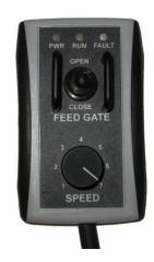
The seven-position "SPEED" control allows the operator to adjust the drop rate while the machine is in operation. The drop rates correspond to 25-175 spheres per minute in 25 spm increments.
