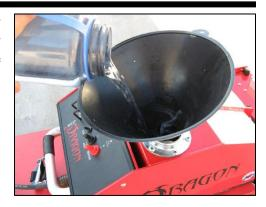
• Fill the glycol tank with undiluted and unused ethylene glycol (anti-freeze).
