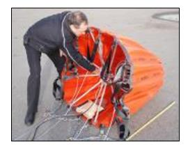
3. Grab the head and pull the suspension lines taut. Tape the lines together in two bunches.
