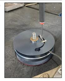
6. Pull out the end of the tripline from the cavity then feed it through the large hole to detach it.
