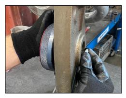
Now that the spring reel is installed into the control head, follow steps 14 - 17 to preload the spring reel.
