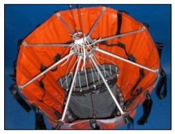
Once the strings are adjusted, fill the Bambi Bucket with water, just below the top of the valve. Check to see if both lips of the valve are matched right across the top. Sometimes, one lip will 'track' slightly above or below the other.
