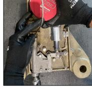
5. Unwrap the remaining tripline from the spring reel then remove the screw and retainer plate from the back of the spring reel.
