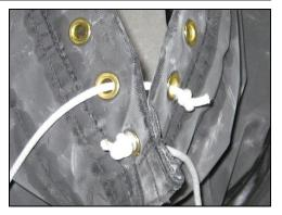
6. Repeat the process with the remaining strings alternating from one side of the valve to the other.
