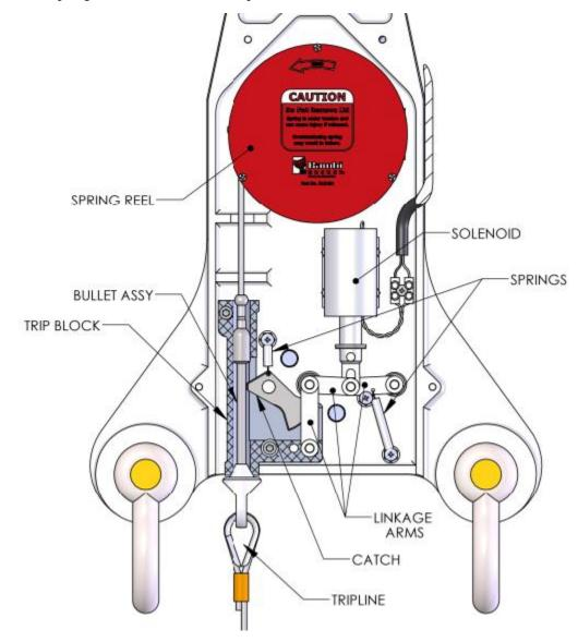
In the middle of the tripline is the bullet assembly. When there is no water in the bucket, the spring reel winds up the tripline until the lower end of the bullet assembly reaches its limit on the bottom of the trip block.
