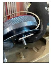
13. Install the nut onto the spring reel arbor while ensuring that the torque plate is still seated properly on the arbor.
