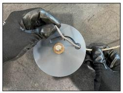
8. (*Tripline*) Insert the end of the new tripline up and through the bottom of the tripblock.
