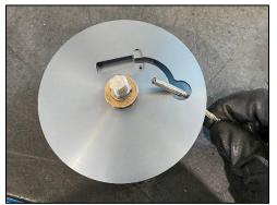
12. Check that the washer and torque plate are installed onto the spring reel arbor, then insert it into the control head so that the torque plate is seated between the tabs on the casting.
