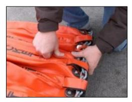
7. Place the control head bag on top of the collapsed bucket.
