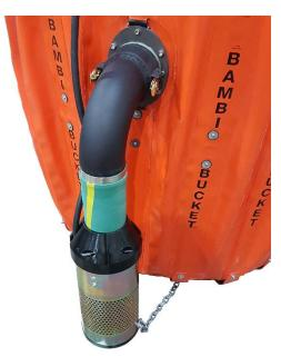
The pump is driven by a 28 VDC electric motor. The motor, impeller and housings are contained within a circular steel filter basket which serves to protect the components from impact damage while also acting as a debris screen.
