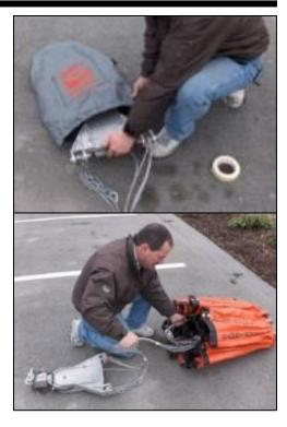
6. Avoid any sharp folds along the base of the shell as this protects the shell from delamination which can occur if the Bambi Bucket is stored for a long period of time.
