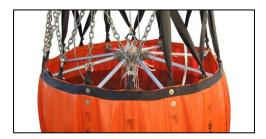
To deploy the IDS on the ground, reach into the bucket, grasp the hub of the IDS and pull outward fully until the two restraining cables from the hub to the lower bucket shell are tight.
