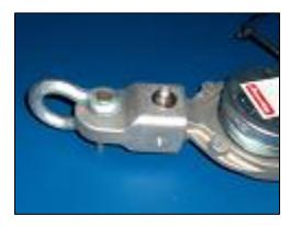
In some cases, where the cargo hook is too large for the standard shackle, a second larger shackle can be used. If the shackle it too large, it may cause the power cable to tangle, pulling apart the break away plug.
