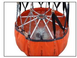
To deploy the IDS on the ground, reach into the bucket, grasp the hub of the IDS and pull outward fully until the two restraining cables from the hub to the lower bucket shell are tight.
