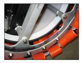
2. Collapse the IDS by pushing the hub into the bucket.
