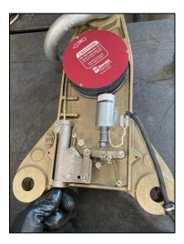
16. Grip the spring reel and hold it in place, then wrap the tripline **counterclockwise** onto the drum of the spring reel **5 revolutions**.
