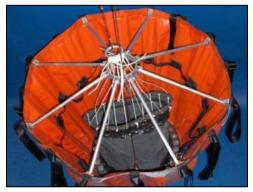
Once the strings are adjusted, fill the Bambi Bucket with water, just below the top of the valve. Check to see if both lips of the valve are matched right across the top. Sometimes, one lip will 'track' slightly above or below the other.
