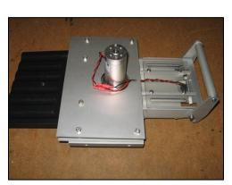
• Loosen the # 8-32 setscrew which secures the agitator cam to the hopper motor shaft.
