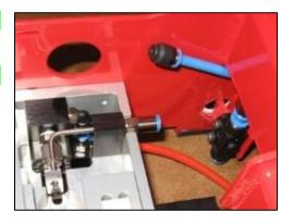
Replace the check valve ensuring proper orientation.
