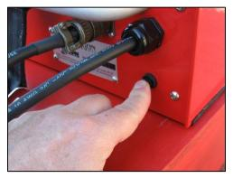
• Switch the "RUN/STOP" switch on the main control panel to "RUN".
