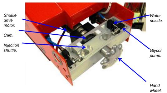
The injection head is the heart of the Red Dragon Dispenser. It is here that the Dragon Eggs are pierced by a hollow needle, injected with a controlled amount of glycol and then ejected from the machine.
