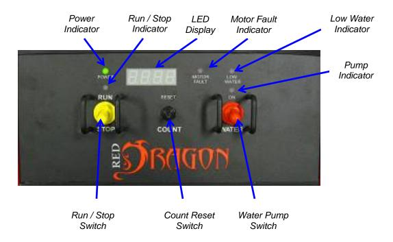
The control panel is the brains of the Red Dragon system. A single circuit board mounted beneath the main control panel contains the microprocessor and all additional components.
