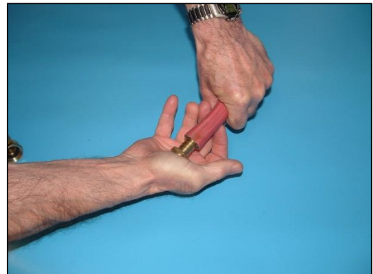
Figure 4-Installing the barbed fitting
