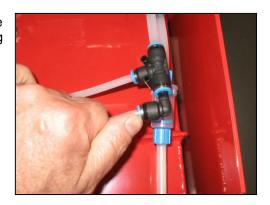
Remove the other end of the discharge line from the water nozzle block inlet.
