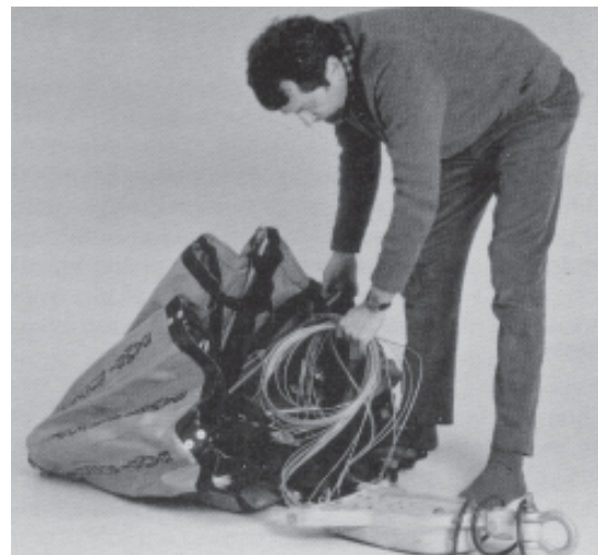
Fig. 9.2: Loop suspension lines and stow inside bucket
