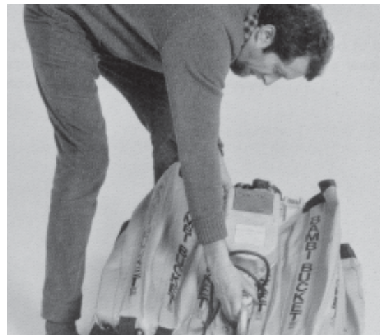
Fig. 9.3: Place control head on collapsed bucket
