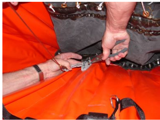
Removing the clevis pin
