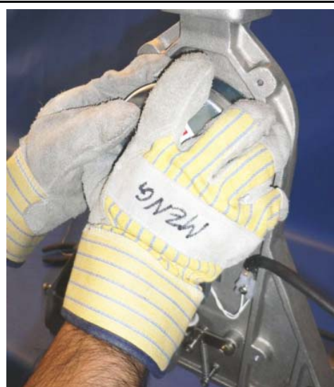
Slowly release the tension on the spring.
