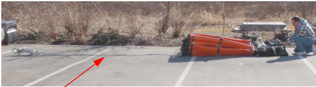
Measuring the bucket. If an attachment is to be used, attach first and then measure to the bottom of the attachment.
