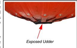
A properly adjusted dump valve will have a maximum of 2" (50 mm) of udder. Too much udder will add to the volume and thus the weight of the bucket. Too little udder will prevent the secondary sealing action and will result in the valve leaking.
