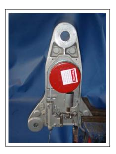
2. If the tripline is not broken above the trip block and the spring reel is functional, push the solenoid up locking the catch open with a bolt or pin and pull the tripline out to its full extent.
