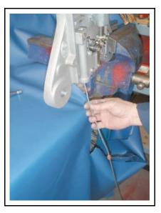
2. Once the tripline has passed through the trip block, bend the end of the tripline into a tight spiral using a pair of pliers.
