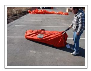
The Bambi bucket carrying bag makes a suitable shipping container when shipping via airfreight. Because of the compactness of the Bambi, many operators carry it aboard the helicopter, at all times, during the fire season. This allows for rapid deployment when required.
