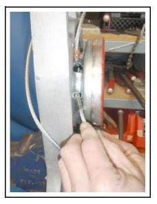
5. Locate the locking finger in the large center hole of the reel. Push the swage on the end of the tripline past this locking finger.
