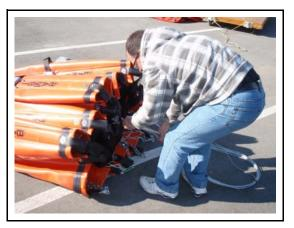
4. Place the head and Firesock on top of the bucket. Using the two straps supplied, strap the bucket to secure.
