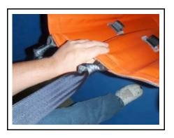
7. The M strap set should now look like this. The suspension line attaches to the top of each M-strap set.
