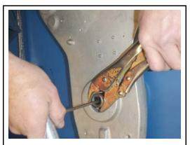
Hold the threaded bolt with an Allen key.
