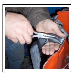
3. Holding the pliers tight, turn your hand clockwise. Repeat the operation until the knot is loose enough to remove the strap.
