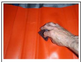
Clean and apply masking tape on the backside of the tear.
