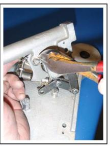
8. Remount the trip block, the spring link clevis pin and the return spring mounting bolt.
