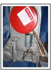
4. Stop spring reel when the openings are at the top.
