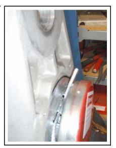
4. Pull 12-14" (30-35 cm) of line from the hole and pull it around the drum in a clockwise motion. Insert the tripline into the small hole to the left of the larger hole, when facing the head.
