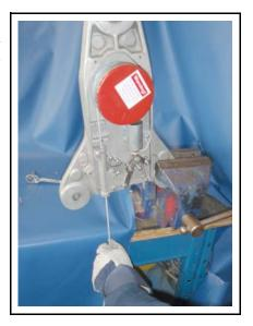
10. Place the bolt or pin to hold the catch in its open position, then pull the tripline out 3-4 ft. and return it to the retract position. Repeat four to five times, then remove the bolt and replace the cover.
