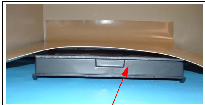
The damaged area should be supported on a flat, solid platform.
