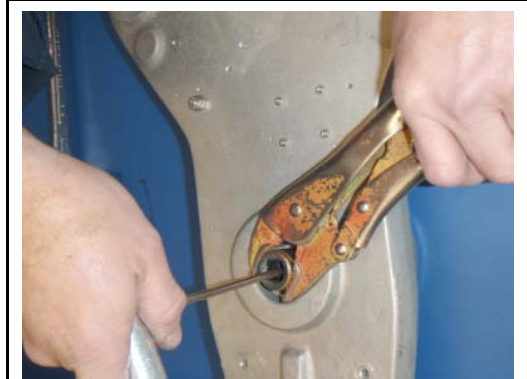
Hold the threaded bolt with an Allen key.
