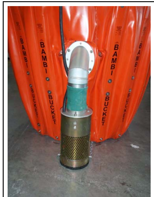
Bambi bucket with PowerFill installed.
