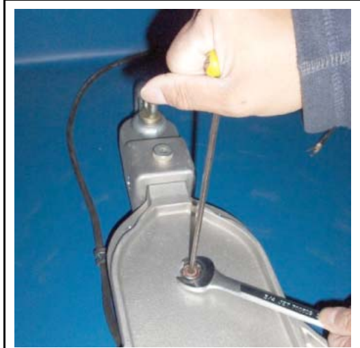
Holding the threaded bolt with an Allen key.
