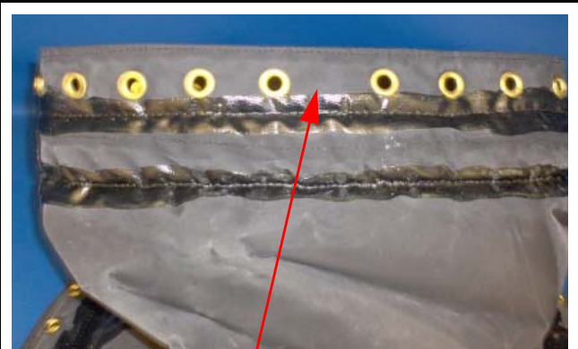
Large gap between grommets shows bolt location.
