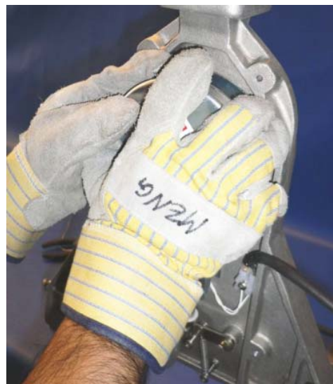
Slowly release the tension on the spring.
