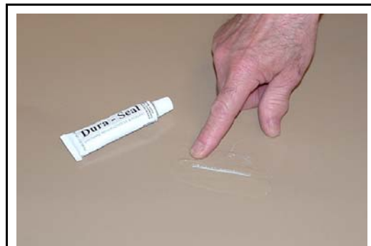
Squeeze glue around tear and spread with fingers.
