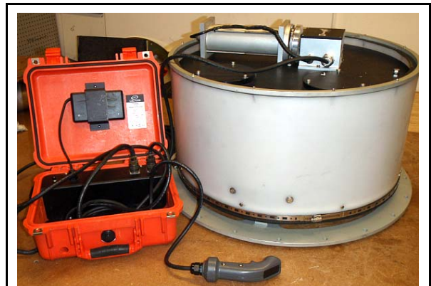
Valve in partially open position and shown with the Bambi Power Pack.
