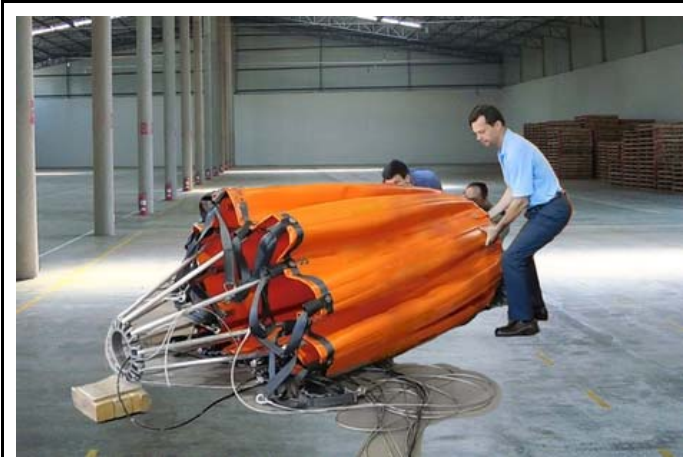
Place the bucket on the blocks as shown and lift.
