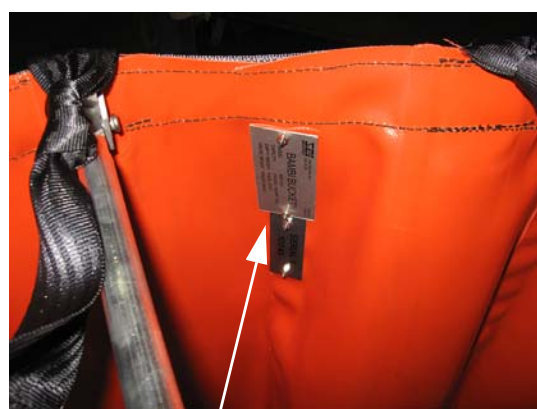
Bambi MAX shell serial number location.
