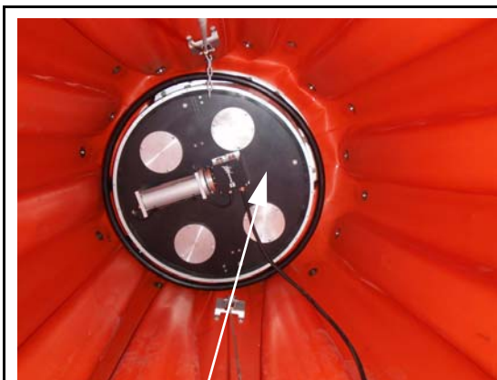
Bambi MAX valve serial number location.
