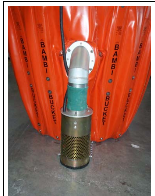
Bambi bucket with PowerFill installed.
