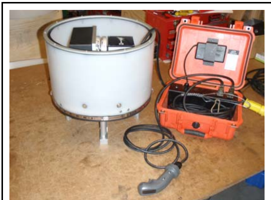
Valve in partially open position and shown with the Bambi Power Pack.
