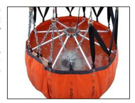
To deploy the IDS on the ground, reach into the bucket, grasp the hub of the IDS and pull outward fully until the two restraining cables from the hub to the lower bucket shell are tight.
