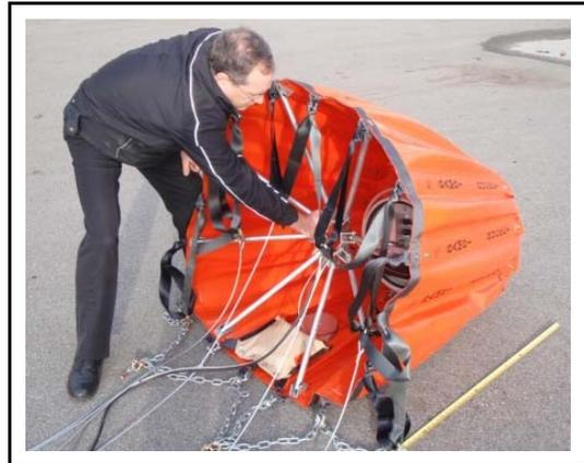
2. Grab the head and pull the suspension lines taut. Tape the lines together in two bunches.
