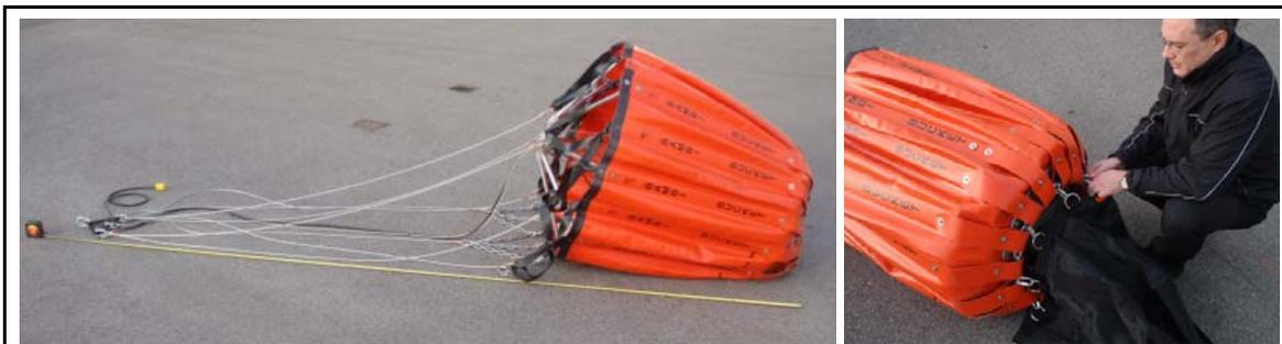
*Measuring the bucket. If a Firesock is to be used, attach first and then measure to the bottom of the sock. See Section 4: Flight Operations for information on how to use the Firesock.*
