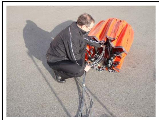
5. Place the head on top of the collapsed bucket.
