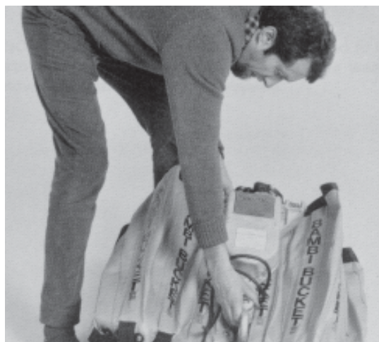
Fig. 11: Place head on collapsed bucket.
