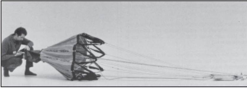
Fig. 2: Measuring overall length of Bambi.
