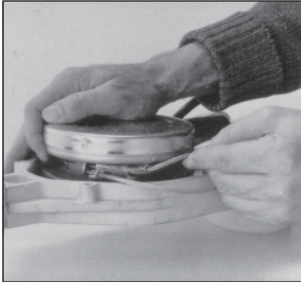
Fig. 28: Insert trip line into small hole.
