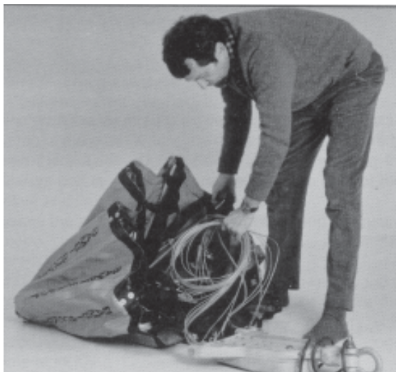
Fig. 10: Loop suspension lines and stow inside bucket
