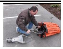
6. Avoid any sharp folds along the base of the shell as this protects the shell from delamination which can occur if the Bambi Bucket is stored for a long period of time.
