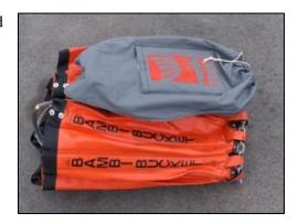
8. Roll the bucket into a bundle and wrap with straps supplied.
