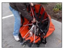
2. Grab the control head and pull the suspension lines taut. Tape the lines together in two bunches.
