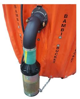
The pump is driven by a 28 VDC electric motor. The motor, impeller and housings are contained within a circular steel filter basket which serves to protect the components from impact damage while also acting as a debris screen.
