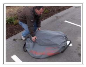
Roll the bucket over and insert the bucket and Firesock into the bag.
