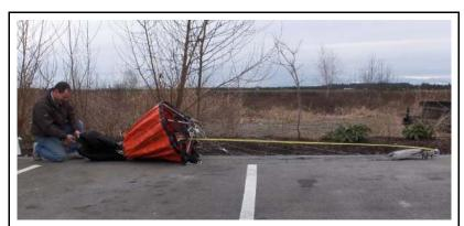
Measuring the bucket. If a Firesock is to be used, attach first and then measure to the bottom of the sock. See Section 4: Flight Operations for information on how to use the Firesock.
