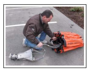
5. Avoid any sharp folds along the base of the shell as this protects the shell from delamination which can occur if the Bambi bucket is stored for a long period of time.
