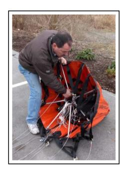
Grab the control head and pull the suspension lines taut. Tape the lines together in two bunches.
