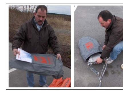
Gather the suspension lines into a coil and stow inside the bucket. Place the control head outside of the bucket to prevent the possibility of the lines tangling.
