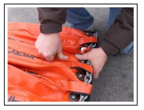
Place the control head bag on top of the collapsed bucket.
