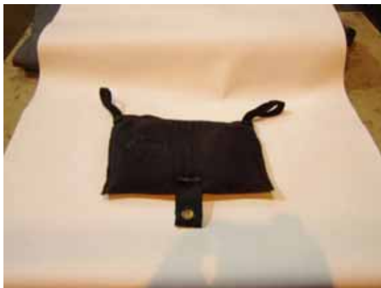
Ballast Bags (used on older models of the Bambi Bucket) are located on the inside of the shell.
