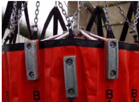
Steel Ballast Bars mounted to the outside of a Bambi Bucket.
