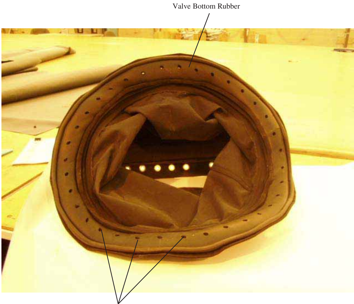
Bolt holes are punched into the neoprene rubber
