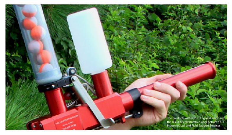
The Pyroshot 'High Speed' is a gas-propelled, triggeractivated Dragon Egg hand-launcher. The Pyroshot HS uses a 5 lbs.  $CO_2$  beverage bottle (or a 20 ounce mini-bottle carried on the belt) to easily launch Dragon Eggs 320 ft.
