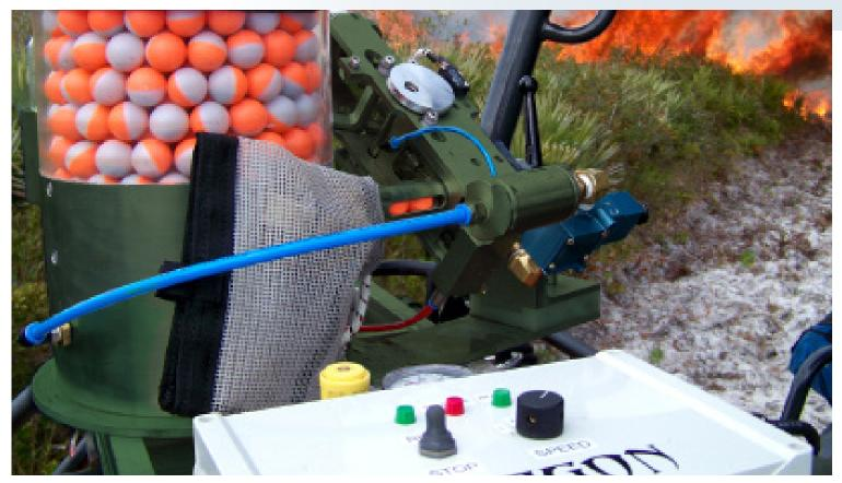
The Green Dragon® is an automated ground launcher designed and engineered for use in wildfire and land management applications such as back burns or prescribed burning. Its design represents a brand new concept for ground ignition applications using CO<sub>2</sub> or compressed air as a propellant and a simple electrically-driven reciprocating feed and firing system. The Green Dragon can be successfully mounted on several ground-based platforms including trucks, boats, ATVs and UTVs.
