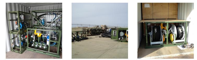
Various nozzles are provided to enable filling of ground vehicles, tanker trucks or small aircraft. Portable secondary containment is provided for each mechanical skid. Flexible hoses are provided to connect the entire system together via manifolds built onto each filling and dispensing skid.
