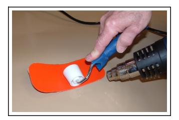
Roll the patch down to fuse it to the fabric, moving roller and gun simultaneously. Repeat on the un-fused portion of the patch. Let the repaired area cool down. Attempt to peel off at the edges with your fingers. If there is even a slight peel, repeat the operation on that small area. Otherwise, the repair is finished.
