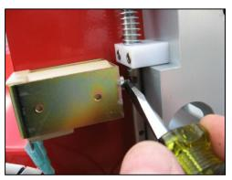
• Clean the sphere paths in the gate assembly using a cloth and a citrus-based cleaner/degreaser such as Simple Green all purpose cleaner.
