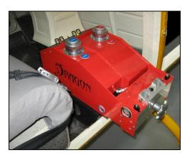
Attach and secure the outlet chute, using a thumbnut and locking thumbnut on each screw. The gold nut must be located on the outside of the injection head, followed by the black nut.
