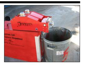
• Place two spheres into each of the cavities of the gate assembly.
