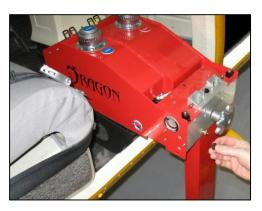
Attach the Y strap by snapping the "Y" end to the holes on each side of the outboard end of the dispenser. Ensure that the strap goes inboard of the exit chute.
