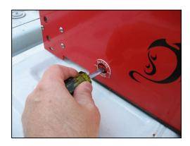
• Check/fill the water storage tank. Secure the filler/breather cap.
