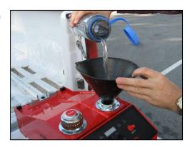
• Check/fill the glycol tank with undiluted and unused ethylene glycol (anti-freeze). Secure the filler/breather cap.
