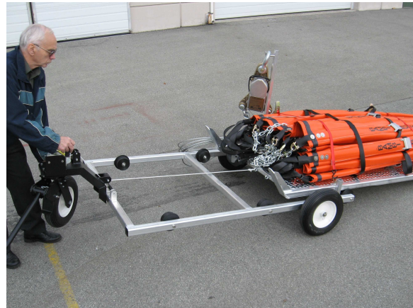
4. Continue cranking until skid is off the cart.
