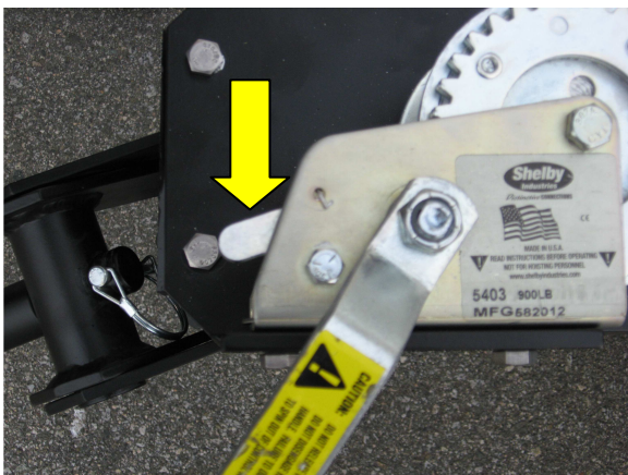
7. Set winch to load position.
