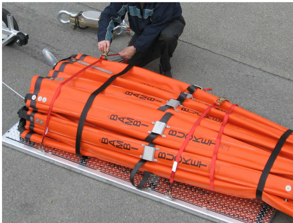
5. Remove straps which secure bucket to skid.
