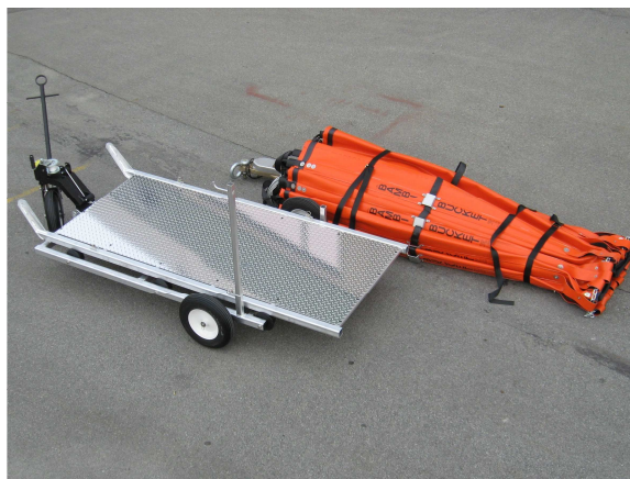
8. Crank winch to put skid on cart.
