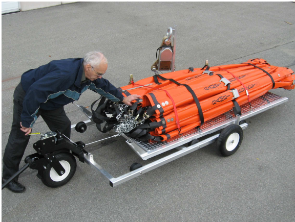
3. While cranking push the skid off the cart.
