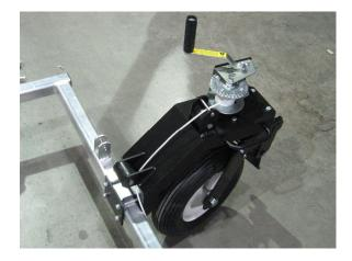
3. Attach front wheel assembly to cart frame at the location marked on the frame.
