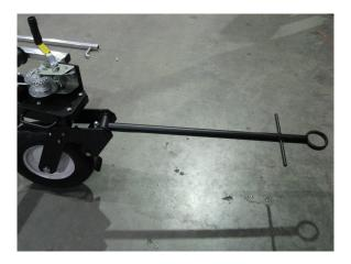
4. Install tow bar into front wheel assembly.
