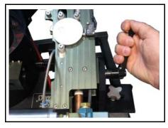
Remove the four socket head cap screws which secure the front plate to the side plates of the launcher.
