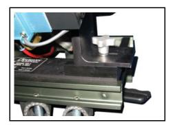
Remove the hopper outlet tube. 4.
