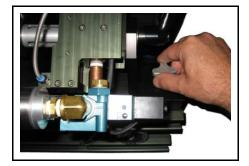
Slide the launcher and slide angle away from the hopper. 3.
