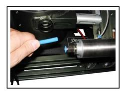
Disconnect the glycol line to the glycol pump inlet valve.
