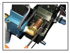
Remove the breech plug and valve assembly and set aside being careful not to damage the valve wires.
