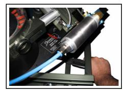
Adjust the elevation of the launcher. 5.
