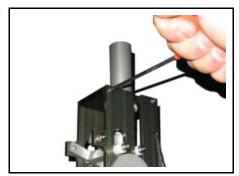
Remove the front plate, front bearing, barrel and barrel spring.
