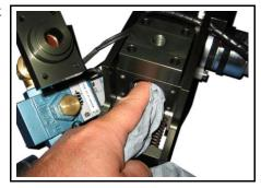
Clean the port in the side of the receiver where the hopper outlet tube mates.
