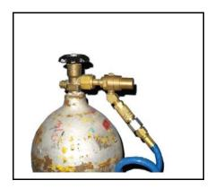
3. Connect the flexible hose to the fitting on the manifold.
