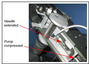
During the second phase of the cycle, the drive cams allow the injection shuttle springs to push the injection shuttle upwards and retract the needle from the egg. The glycol pump returns to its neutral position and recharges with glycol for the next cycle.
