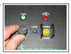
Adjust the pressure regulator to give the desired range. Pull up on the locking ring of the pressure regulator before attempting to rotate.
