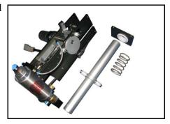
Wipe out the inside of the front bearing and receiver bearing with a cloth. The bearings are self-lubricating and should not be oiled.
