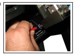
Disconnect the electrical connection to the launcher.
