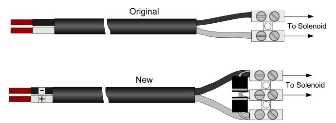
Field replacement of an unpolarized head lead wire with a new-design head lead wire is accomplished by removing the existing wire and its 2-position wiring terminal from the head cavity and installing the new-design head lead wire in its place. The new-design head lead wire integrates a mounting bracket and a strain relief provision. Polarities are of no concern when connecting the solenoid wires, and no modifications to the head are necessary.
